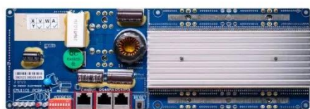
RS485 Communication between battery and inverters Band rate 9600ps
